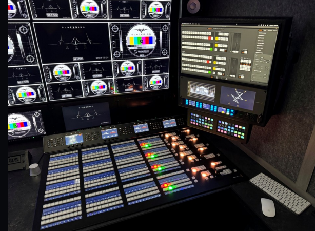
ATEM 4 M/E CONTROL AND AUXILIARY INTERFACE
